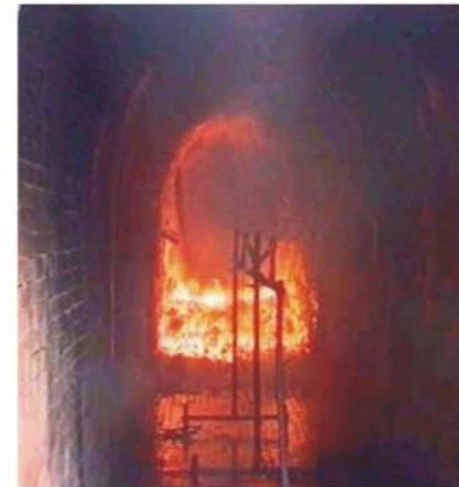
Extinguishing mine fires using water mist
