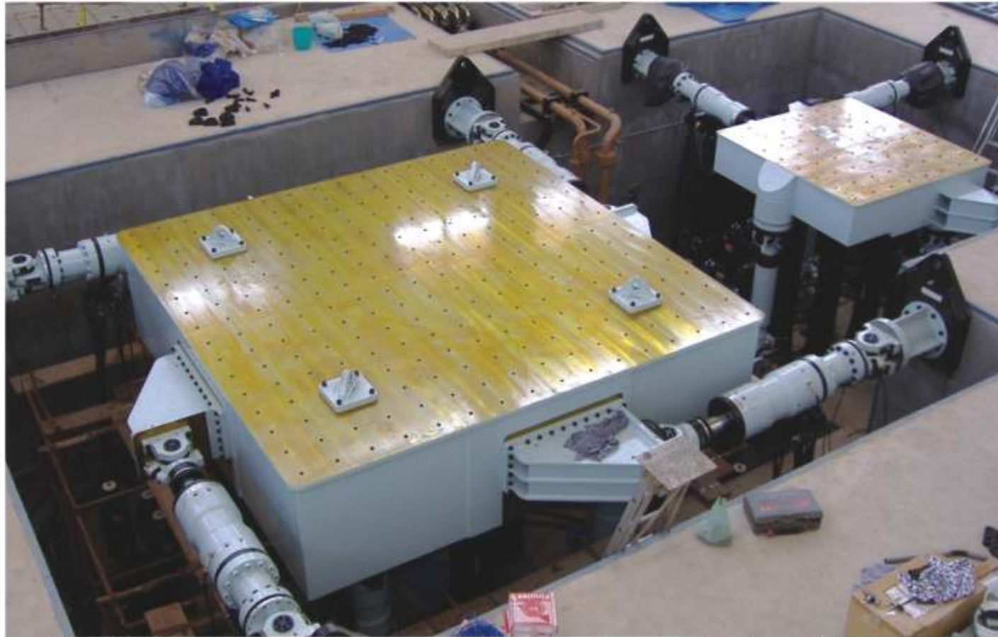
Shake Table with synchronous and asynchronous operation at the advanced seismic testing and research laboratory, SERC, Chennai
