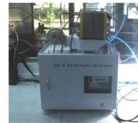
Self-supported 300 W Polymer Electrolyte Fuel Cell System
