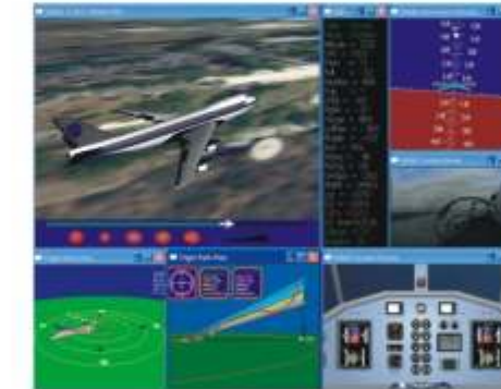
NALVAS showing the capability for aircraft models with ILS operation
