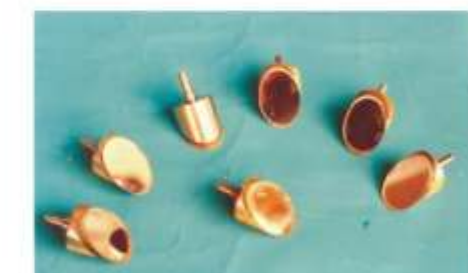
Mirrors for video imaging inside a nuclear reactor
