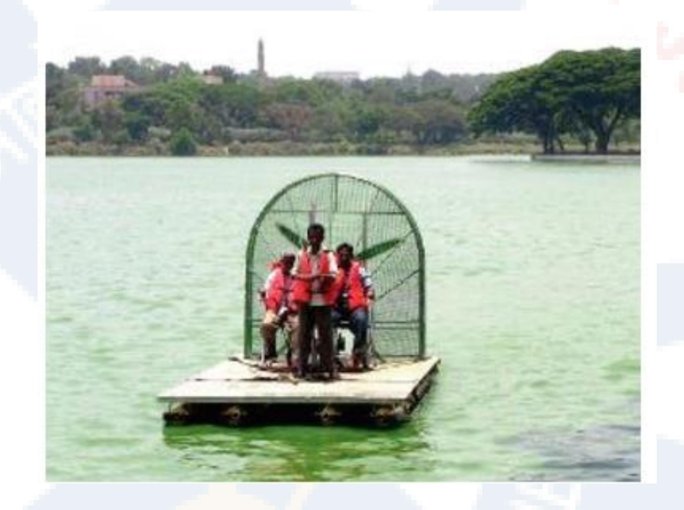
"The airboat will have an air propulsion system which will push it forward. The boat will also have a flat bottom. This kind of boat is ideal for cleaning water bodies. The boat can be pushed into the water and can be scooped out easily. Besides, they have good buoyancy," said NAL chief scientist S Selvarajan.
