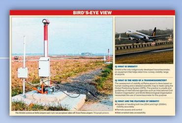
"A transmissometer has been installed adjacent to the runway near the touchdown point for flights," said airport assistant general manager (air traffic management) Santosh Kumar. "It has three components - a sensor, a receiver and a transmitter. There is a gap of 30m between the receiver and transmitter. The censor records visibility readings and the data is continuously sent to the air-traffic controller."
