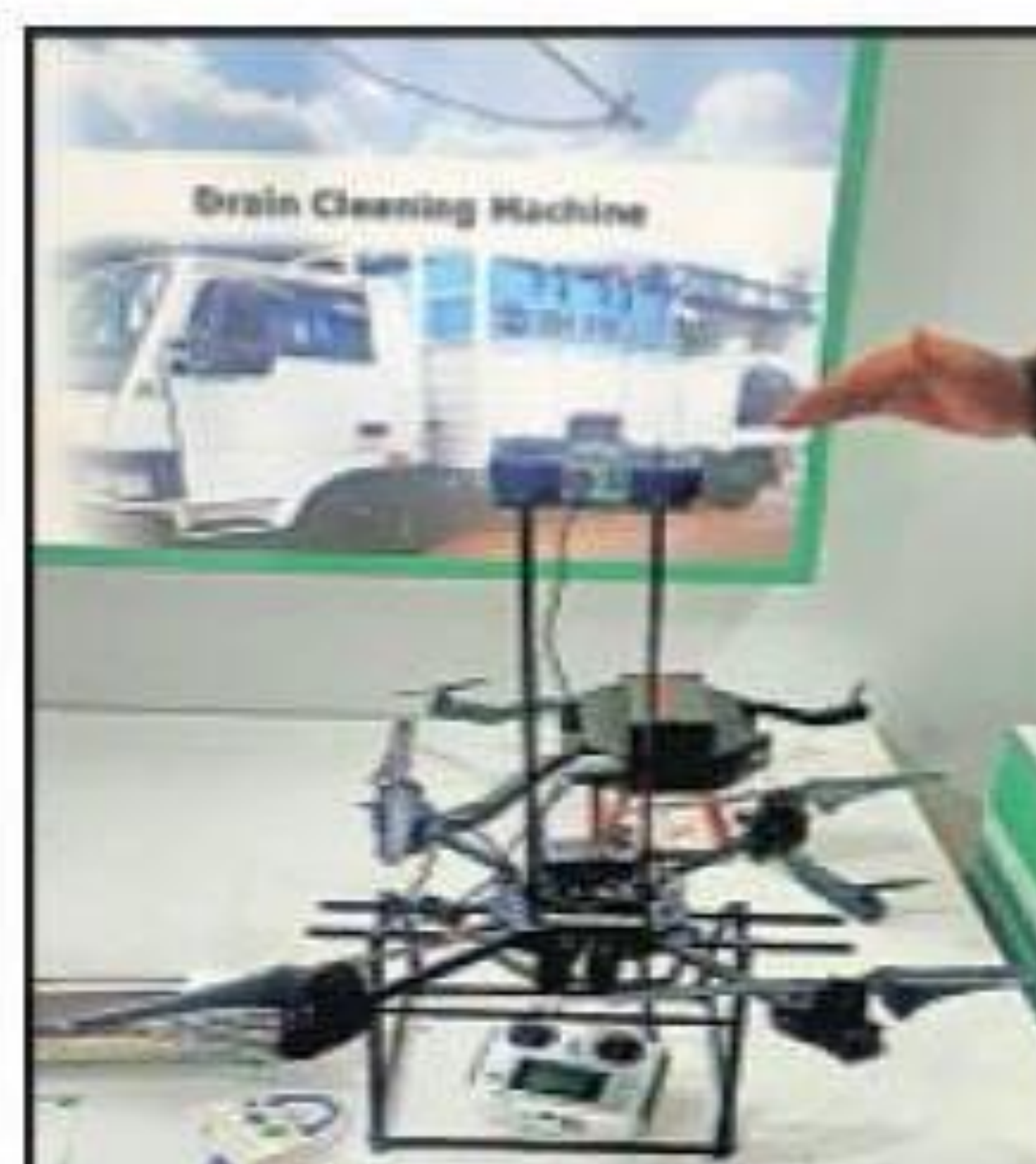
Unmanned Aerial Vehicle (UAV), a Flying Air Quality Laboratory developed by NEERI. (Pic by Satish Raut)
