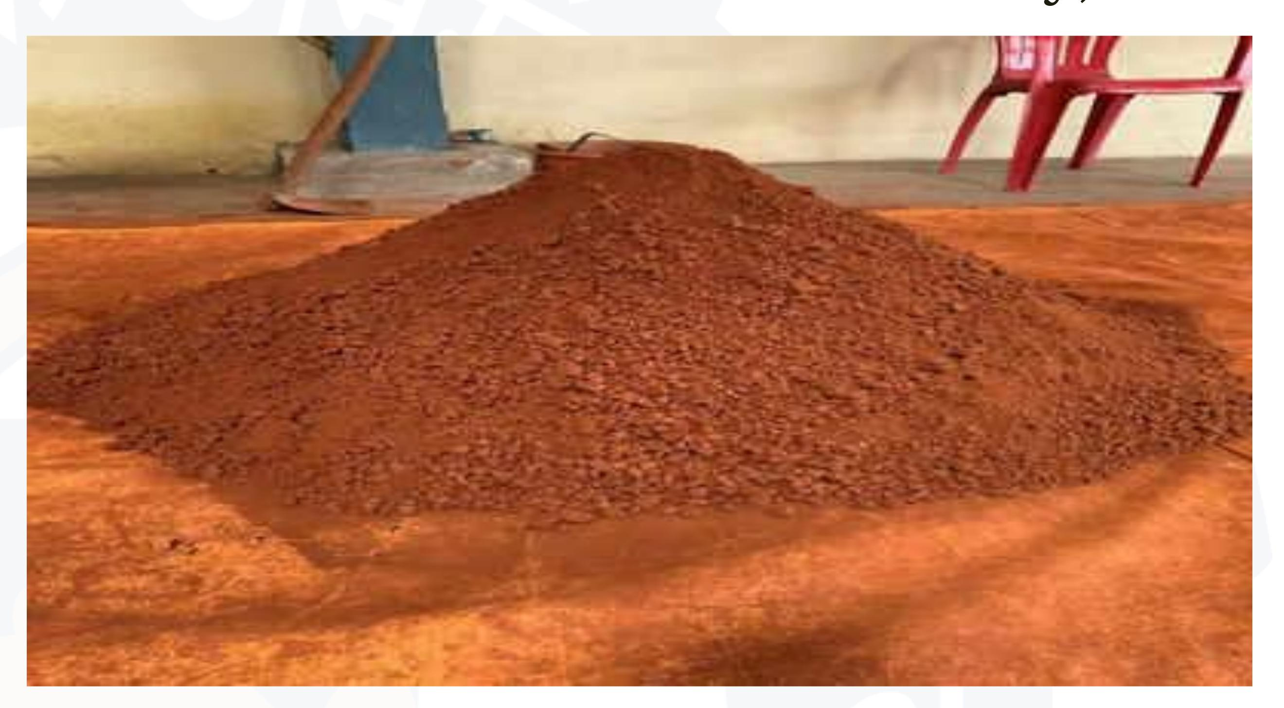
An industry produces more than one tonne of red mud to get one tonne of alumina. Huge amounts of red mud get deposited in the premises of aluminium companies across the world. It has now become a headache for industries to manage the by-product. If the by-product gets into water resources, water gets contaminated. It also affects agriculture too because it is alkaline in nature, said the official sources.
