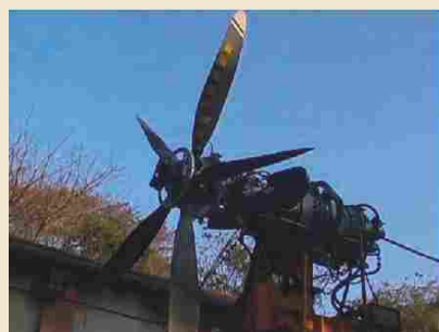
Fig. 1.8: PT6A-67A engine and MT Propeller mounted on the Engine test rig
