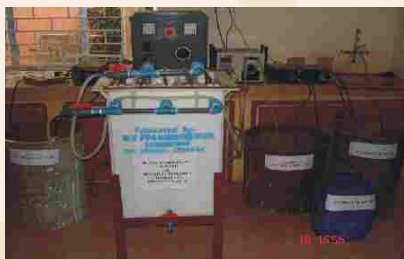
Fig. 1.40: Demonstration unit for Electrolytic reduction
