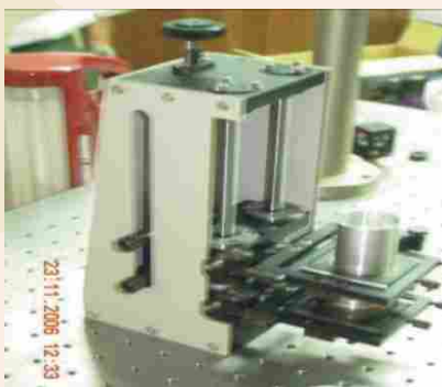
Fig. 1.29: Complete alignment set-up for multi-stage depressed collector
