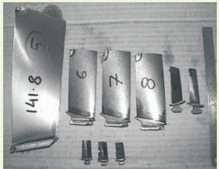
Compressor blades with damaged tip of FRB-2, GGRB-1, GGB-4, GGB-8 and GGB-9
