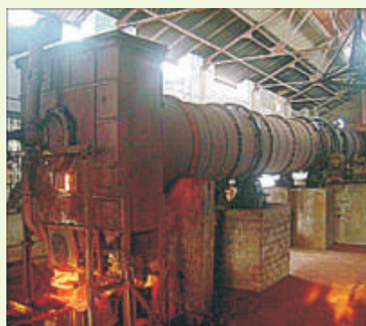
Activation of chromite overburden in Rotary Kiln
