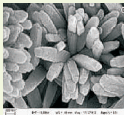
SEM micrographs of the titania films showing rod like structure
