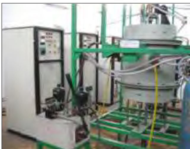
Fig: 1.56 a 50 kW arc plasma reactor
