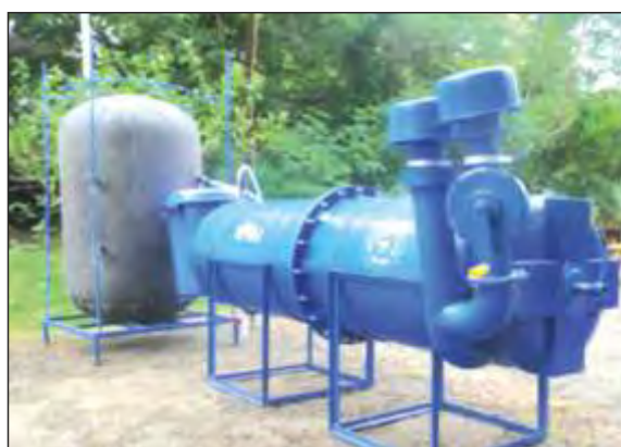
Fig:1.42 The commercial anaerobic treatment system cum biogas plant for household biodegradable wastes
