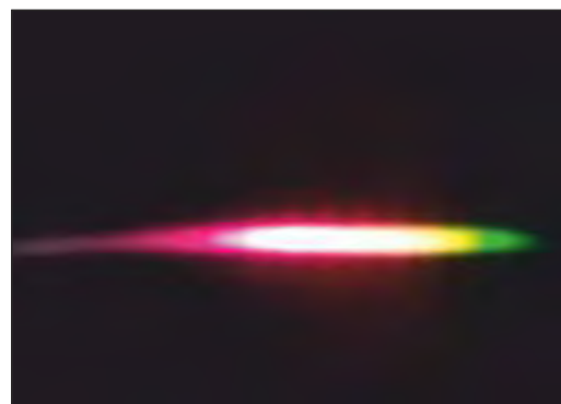
Fig: 3.2b Output of developed Supercontinuum Laser (White laser covering broad wavelength)
