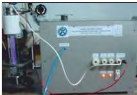
Fig: 1.81 Discharge view of mercury free plasma based water purification system
