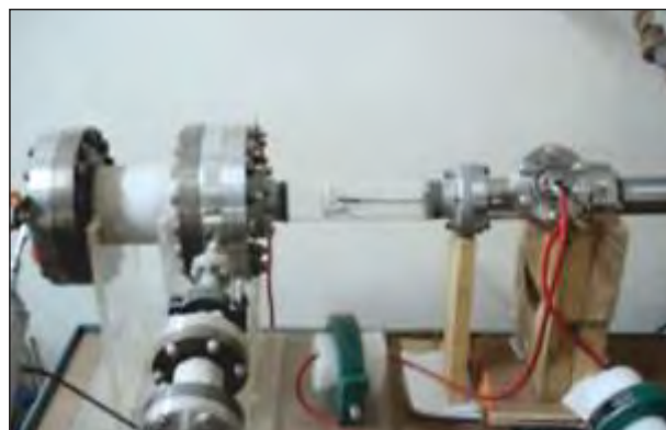
Fig: 1.84 A self-breakdown based single gap plasma cathode electron (PCE) gun
