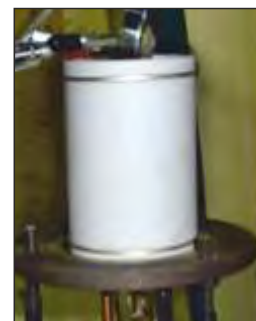
Fig: 1.82 Developed 25kV/5kA Sealed-off PSS
