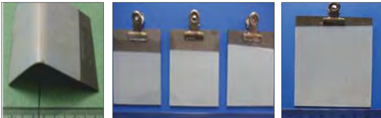
Fig: 1.52 \text{TiO}_2 coating on steel developed- 1200 hrs. salt spray test, explore to 500^\circ\text{C} and 90 degree bend test
