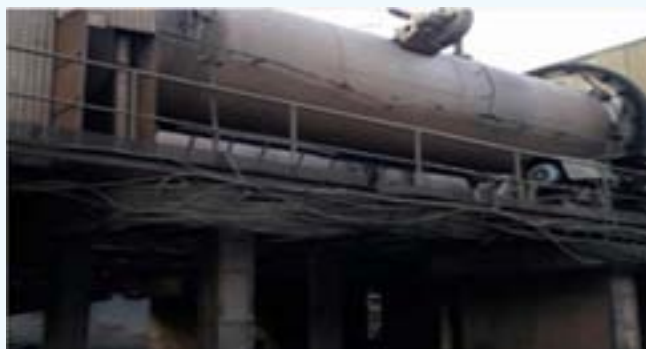
Fig: 7.10 View of 50 TPD capacity commercial DRI Rotary kiln used for metallisation of ilmenite
