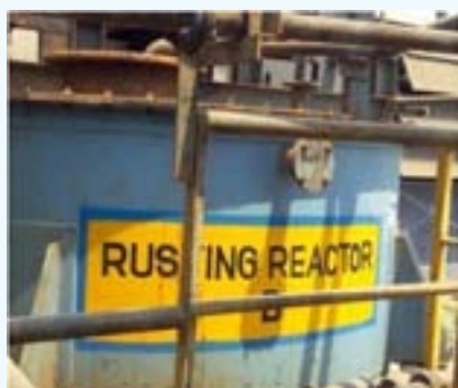
Fig:7.11 Photograph of 5 tonnes /batch rusting reactor
