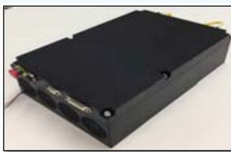
20W High Power Erbium Doped Fibre Amplifier (HP-EDFA) Unit
