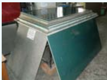
Hybrid green composites for possible use in architectural partition panels
