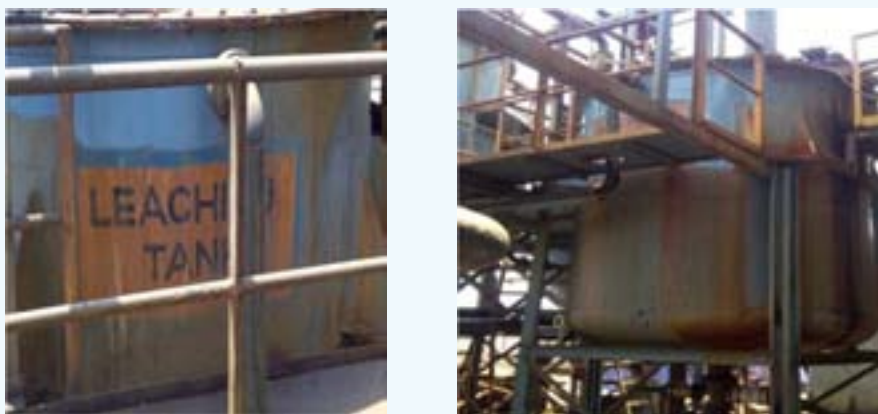
Fig:7.12 Photograph of 2 tonnes/batch leaching reactor
