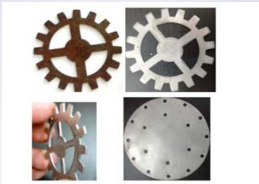
Fig. 8.3.16. Electroless RGO-Ni nanocomposite coated components
