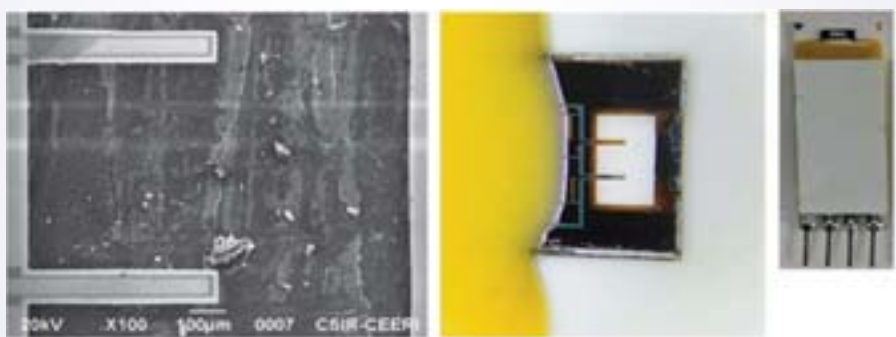
Fig.5.8. (i) SEM image of the micro cantilever based sensing platform (ii) Final two deliverable prototype (close-up view) (iii) Final deliver prototypes
