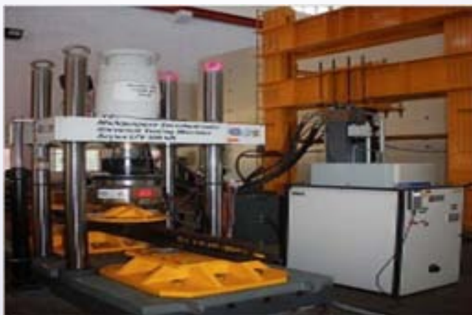
Fig. 5.21. Fatigue life evaluation on welded rail joints
