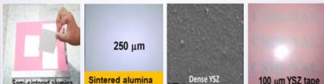
Fig. 8.3.21. Photographs showing the free standing ceramic tapes of alumina and YSZ along with the dense microstructure of YSZ
