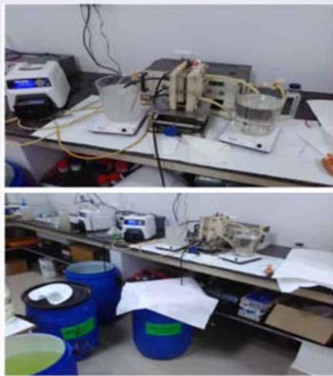
Fig.8.3.17. Test setup for validation of electrolytic-membrane process
