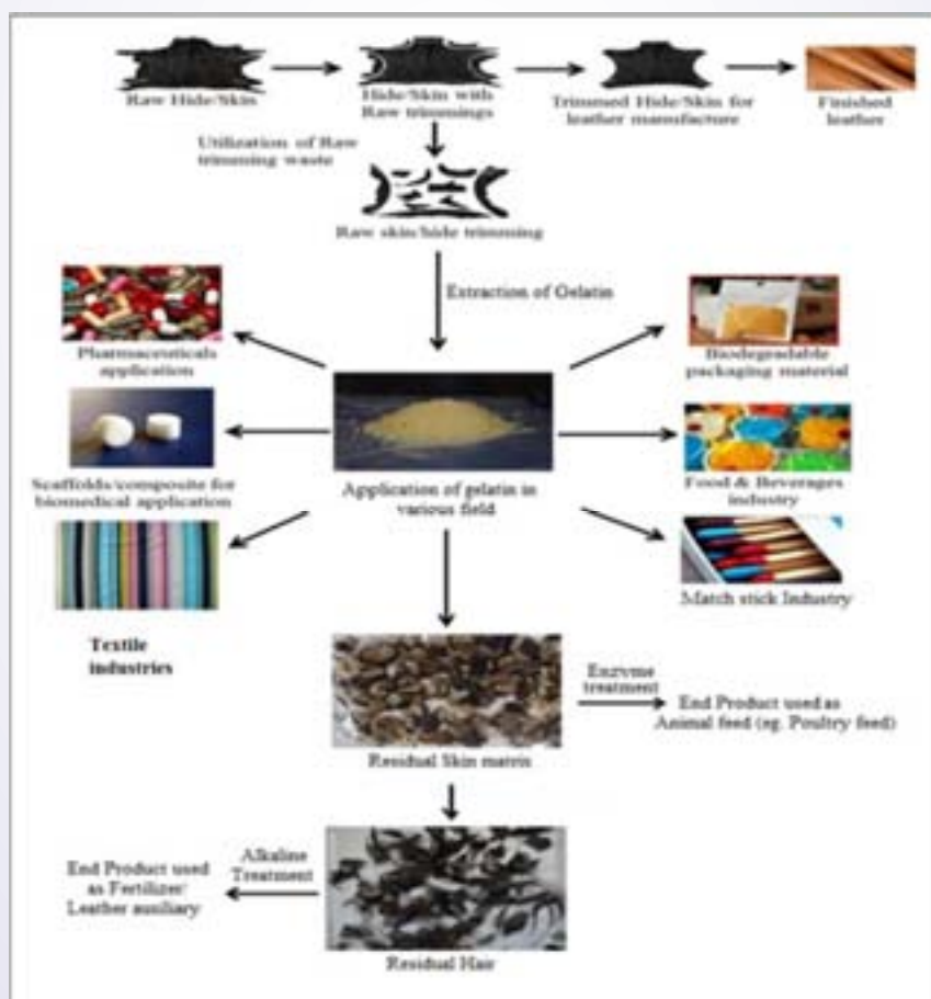
Fig. 8.2.3. process for extraction of gelatin and protein hydrolysate for leather waste
