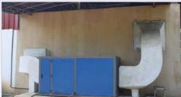
Fig. 7.18. An innovative 'Refrigeration Adsorption Dehumidified Drier' for the low temperature drying of indigenous fruits and vegetables
