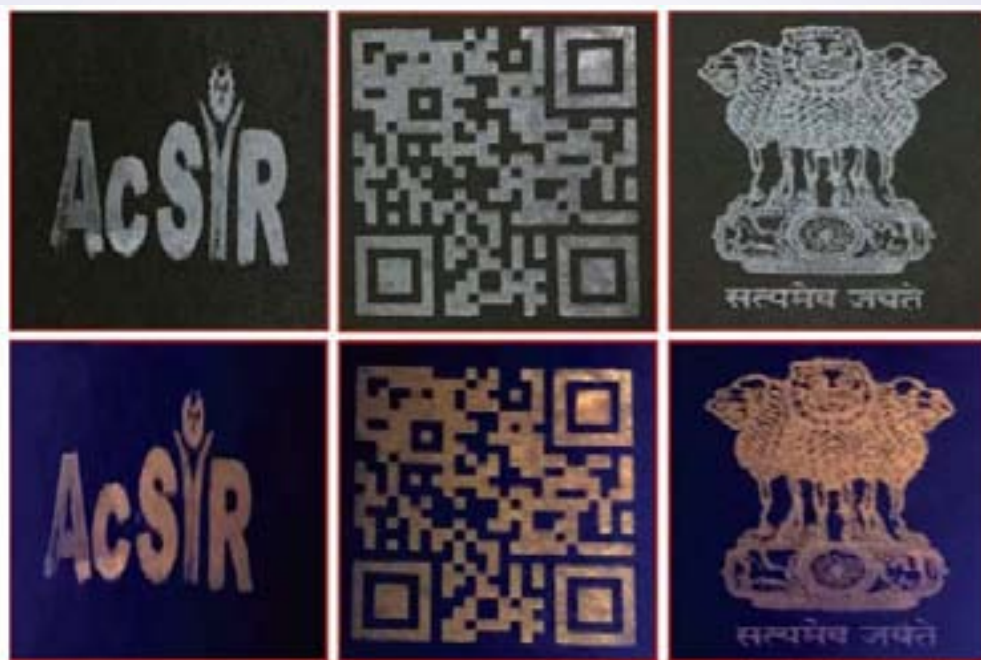
Fig.8.5.9. Prints Using The New Security Ink Appear Differently Under Normal Light (Upper figures) And Under UV Light (lower figures)
