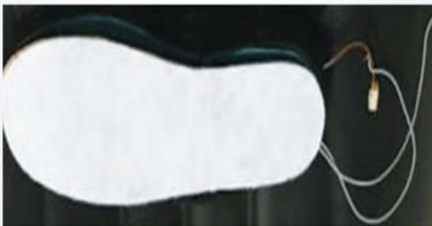
Fig.8.5.3. LTCC/ thick-film hotplate integrated warm-insole
