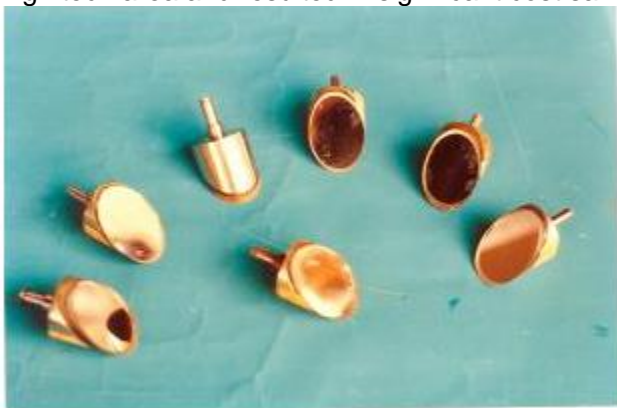
Mirrors for video imaging inside a nuclear reactor
