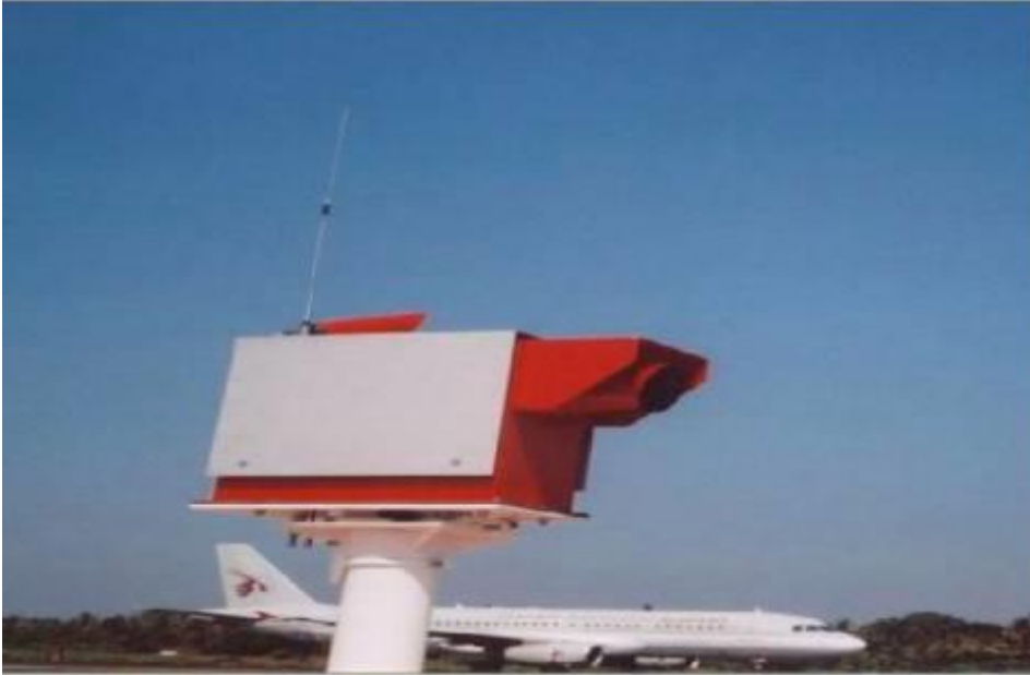
Automatic Visual Range Assessor at Cochin Airport
