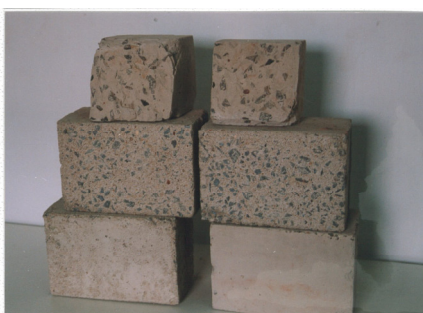
Cement free concrete blocks of fly ash
