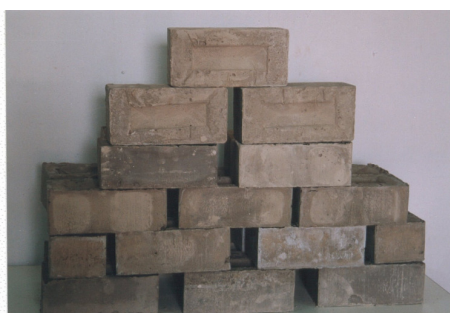
Cold setting building bricks with 95% fly ash
