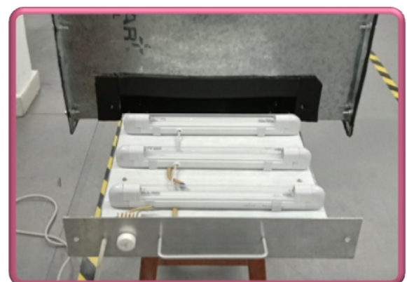
Figure 16 :UV-C retrofit module
