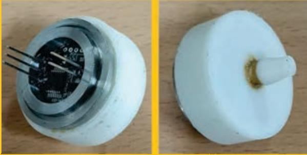
Gauge pressure sensor with SS diaphragm for measuring the pressure range from  $\pm 5$  kPa to  $\pm 100$  kPa.
