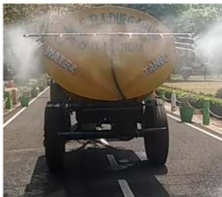
*Tractor operated road disinfection spray system*
