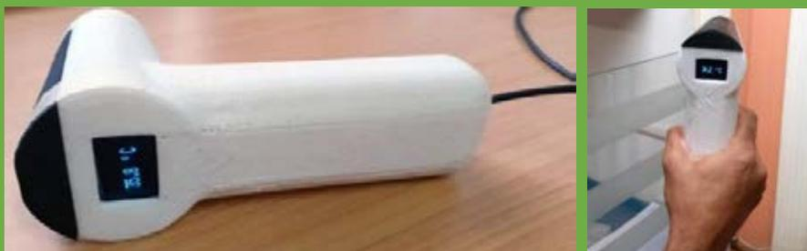
The handheld digital IR thermometer is developed by NCL's Venture Center Incubate, BMek. For the non-contact thermometer, mobile phone or power banks can be used as a power source. Prototype device is currently being used at NCL gate and by Pune Police for screening purposes.
