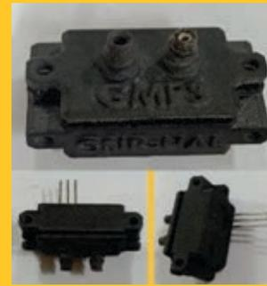
True differential pressure sensor with silicone diaphragm for measuring the pressure range from  $\pm 200$  Pa to  $\pm 2$  kPa
