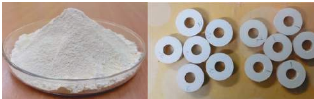
Fig. 5.4.1: PZT powder and fabricated PZT rings prepared at CSIR-NAL team, for accelerometer applications
