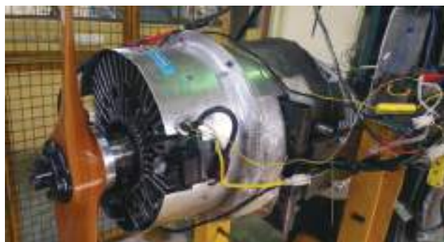
Fig. 7.20: 30 hp Wankel engine in the Test Rig
