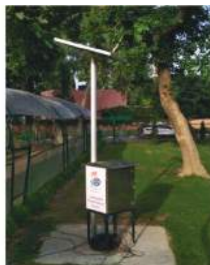
Fig.7.27: Unattended Seismic Ground Movement Detection System installed at CSIR-CSIO campus
