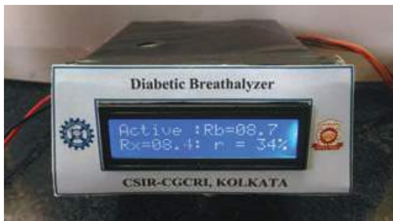
Fig. II.6.14: Test prototype capable of detecting 1 ppm, 2 ppm and 5 ppm acetone in air
