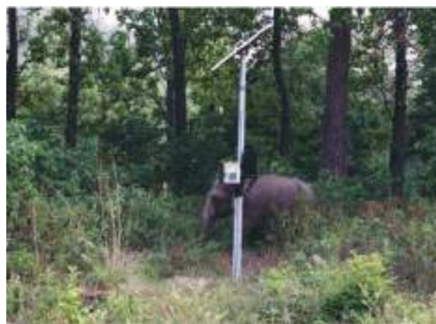
Fig. 7.30: CSIR-CSIO Intelligent Seismic Sensing System deployed at site
