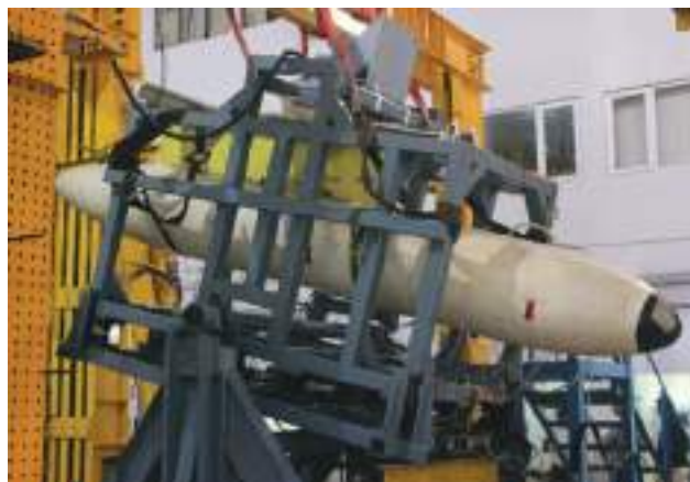
Fig. 6.4.4: Crucial Qualification test on the fuel drop tank
