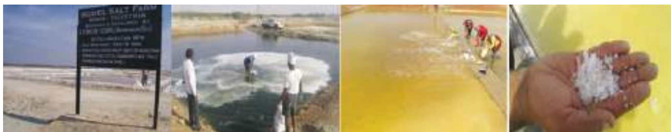
Fig. II.6.8: Process for high purity solar salt production
