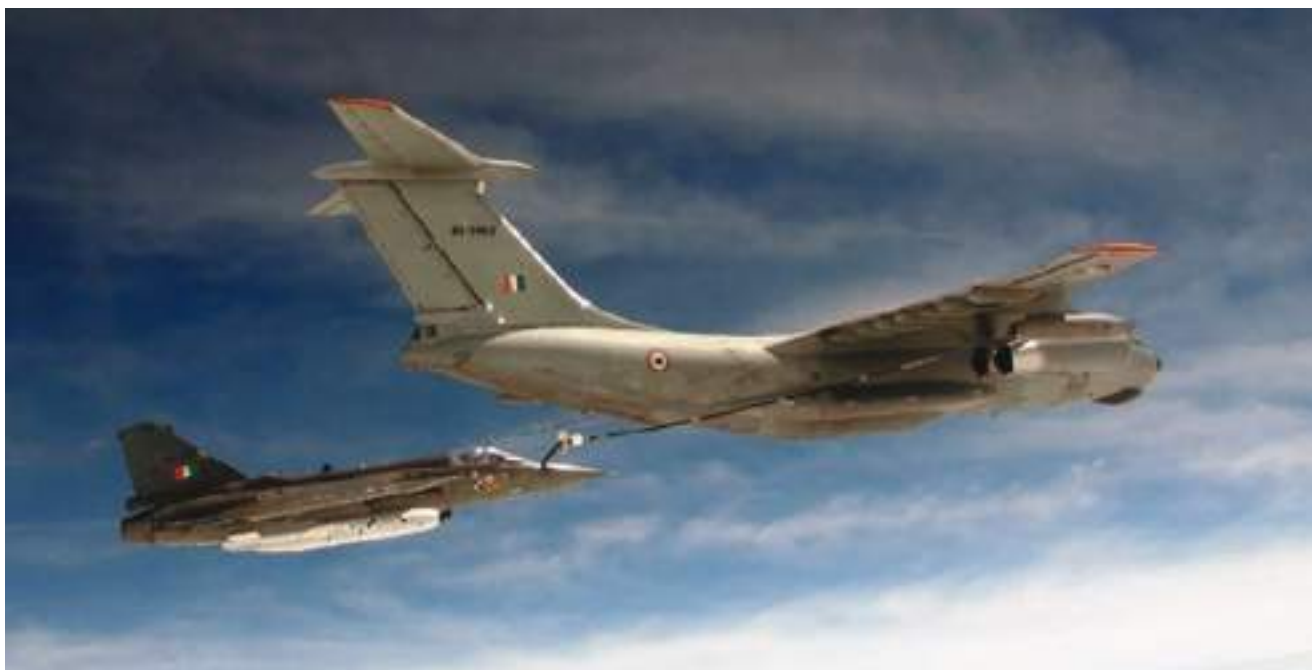
Fig. 6.3.3: Control laws successfully flight-tested for air-to-air refueling
