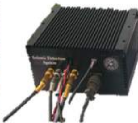
Fig.7.27: Unattended Seismic Ground Movement Detection System installed at CSIR-CSIO campus
