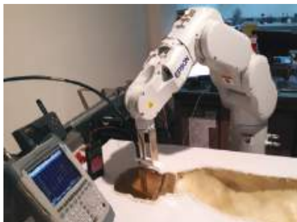
Fig. 7.14: SAR measurement setup at CSIR-NPL
