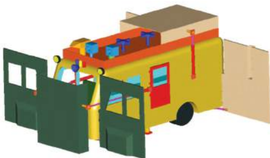
Fig.11.1.19.1: Proposed four-wheeled-drive and three degrees-of-freedom compact armored vehicle with expandable provision
