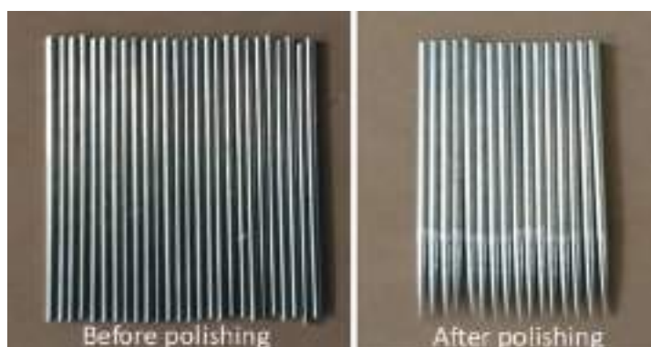
Fig. 6.1.1: Medical grade SS surgical needles before and after electropolishing
