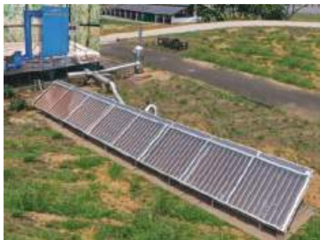
Fig. 9.6: Solar biomass hybrid dryer for drying of fish/spices
