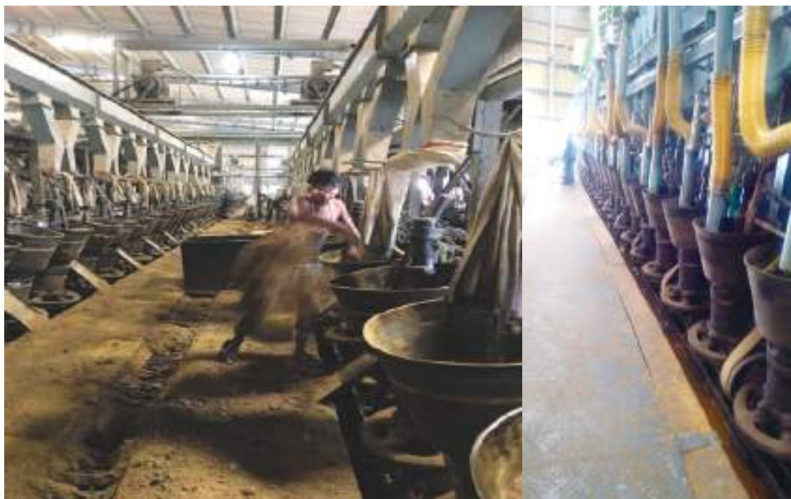
Fig. II.6.17: Automation of Ghani Operation through Vacuum Conveying System'
