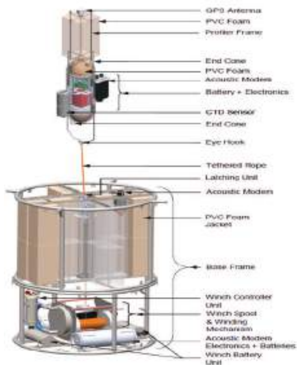
Fig. 7.29: Seabed unit with profiler unit
