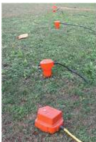
Fig.7.27: Unattended Seismic Ground Movement Detection System installed at CSIR-CSIO campus
