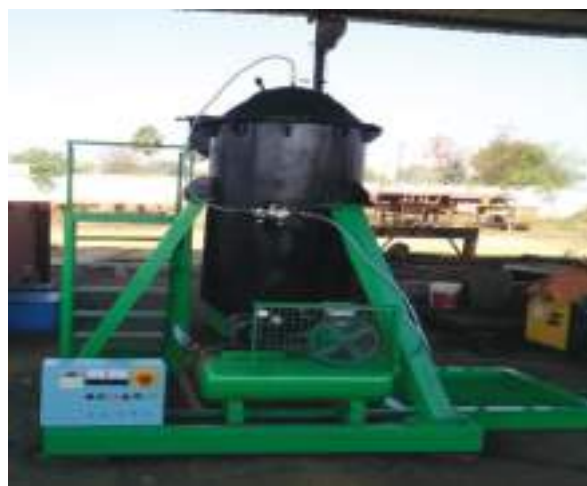
Fig. 6.2.1: CSIR-CIMFR CROW model Coal reject/low grade Coal-biomass based Rural Bio-methane Reactor
