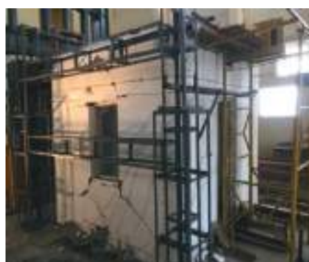
Fig. 5.4.3: Full-scale retrofitted confined masonry building subjected to lateral cyclic load
