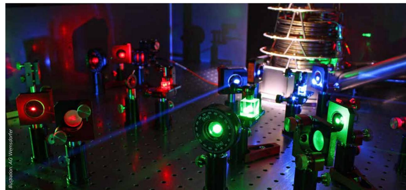
*Optical structure of a laser system. This is used to read out quantum states based on imperfections in diamond.*
