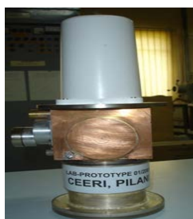
2.6 MW magnetron at it testing in LINAC System
