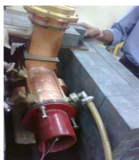
2.6 MW magnetron at it testing in LINAC System
