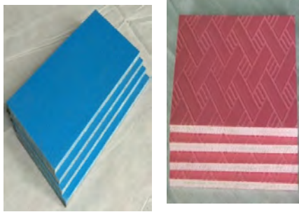
Hybrid green composites of different texture / surface finish
