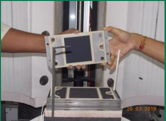
Planar anode-supported single cells (TRL 4 -5) SOFC
