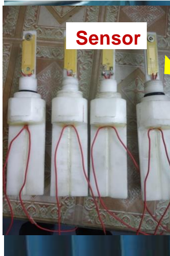
On-site installation of low ppm moisture sensor and digital meter for online measurement of moisture in transformer oil
