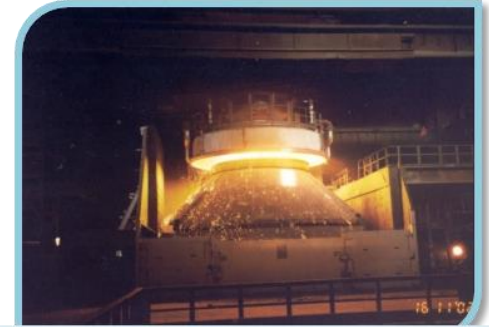
MgO-C Refractory in application at Vizag Steel Plant
