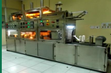
CGCRI designed Lithium Battery Separator fabricator (TRL-4)
