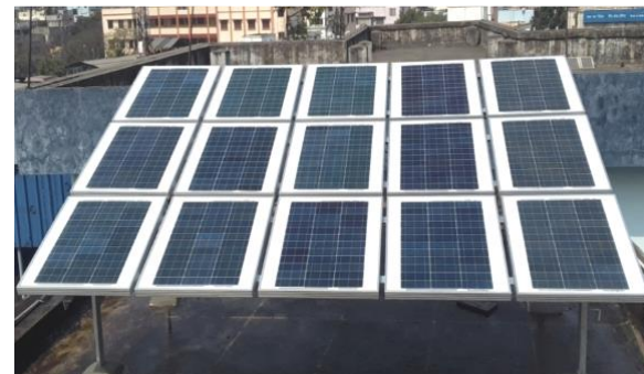
Fabricated solar panels using sol-gel based AR cum hydrophobic coated solar cover glasses
