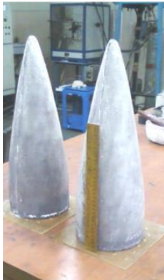
Reaction Bonded Silicon Nitride Missile Radome
