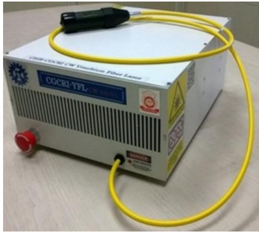
Prototype Laser Module: Power 60 W/100 W and Beam quality M^2 < 1.1
