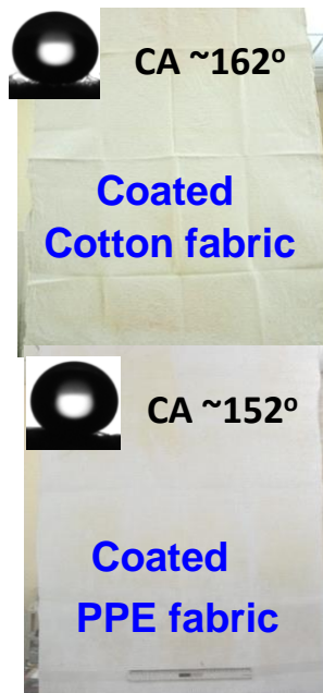
Superhydrophobic and antimicrobial sol-gel based coatings on fabrics
