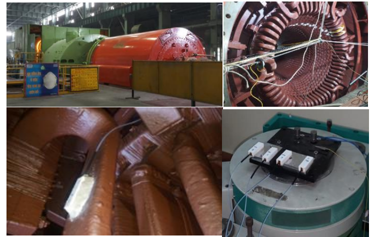
Stator end-wind vibration monitoring: power generators
