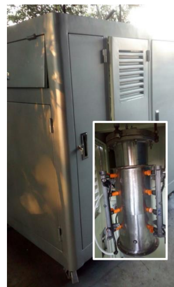
Prototype with Capacity of 1 Nm 3 /h of hydrogen delivery @99.95% purity. Inset a novel
