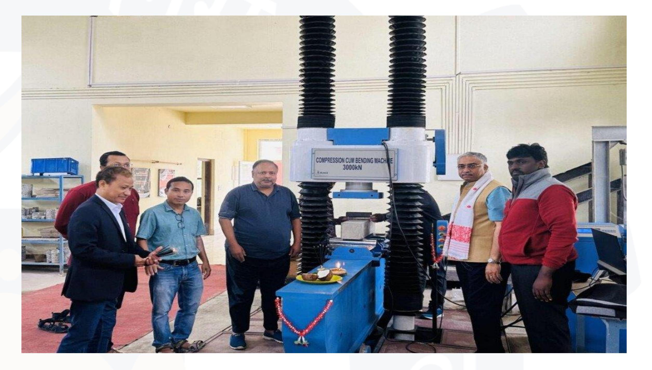
An official stated that the main objective of the facility is to test the structural behaviour of normal and deep beams, steel and concrete columns, trusses, arches, bearing plates, girders, precast tunnel lining units, sleepers, rails, etc.
