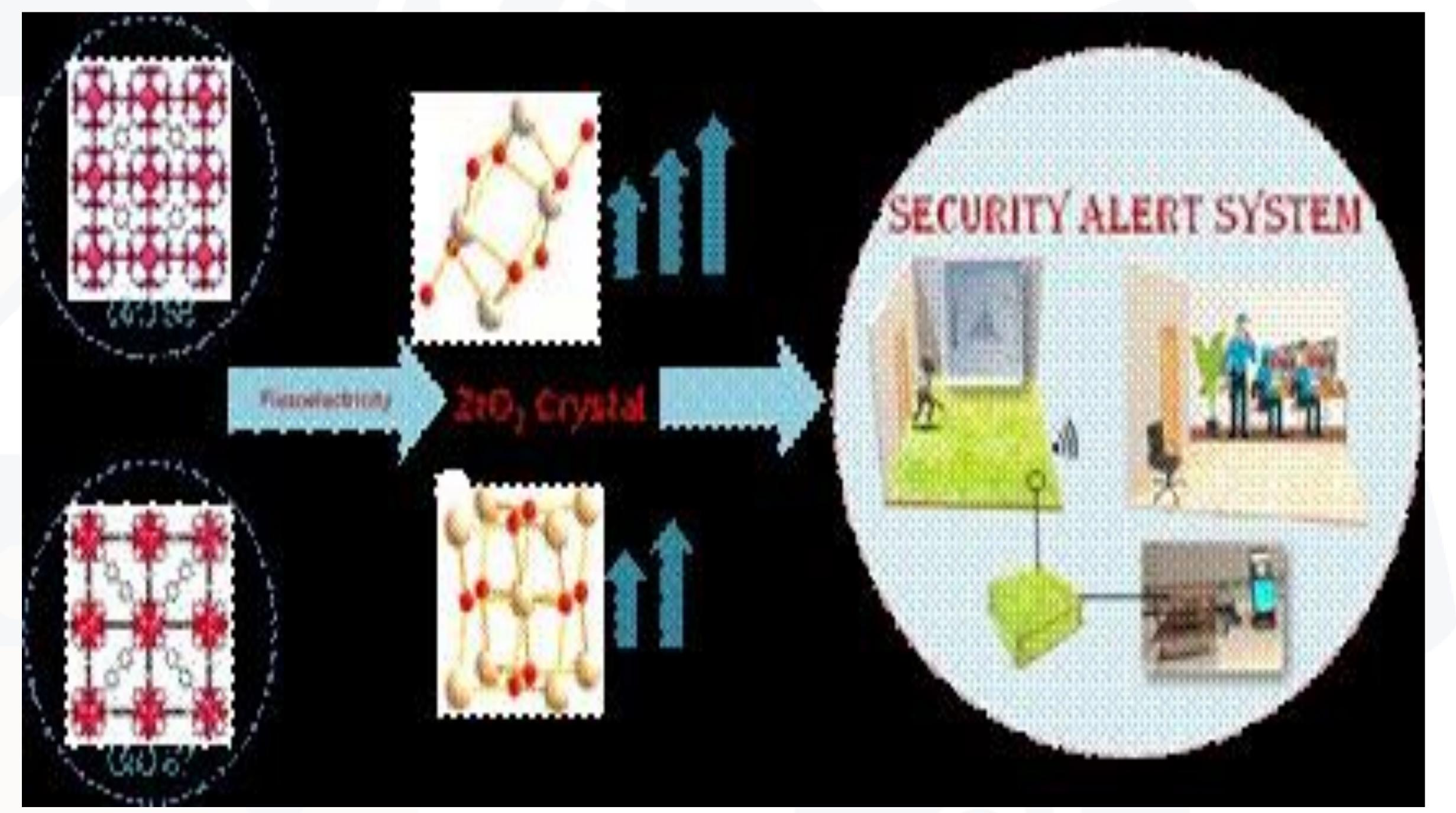
system based on piezoelectric polymer nanocomposite. This development was based on the finding that metal oxide nanomaterials with appropriate crystal structure and surface properties when used as fillers in a polymer composite lead to a significant enhancement in the piezoelectric response.
