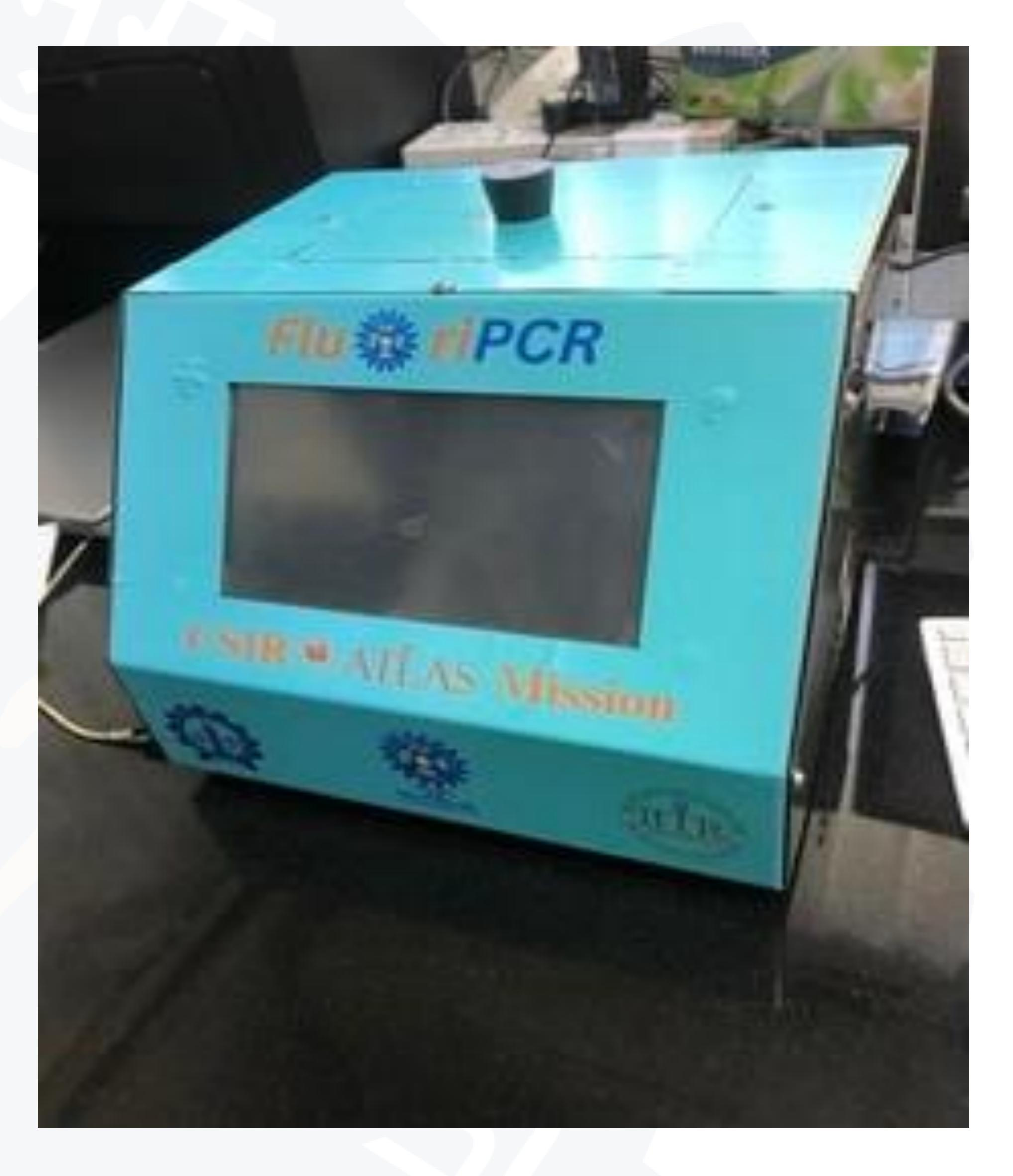
CSIR-IITR has tested FluoriPCR for identifying mixing in meat products and the authenticity of meat species. Buying equipment for carrying out these tests is generally expensive and costs about ₹35 lakh collectively. On the other hand, this device can be made available at ₹1-1.5 lakh, a scientist involved in the innovation process said.
