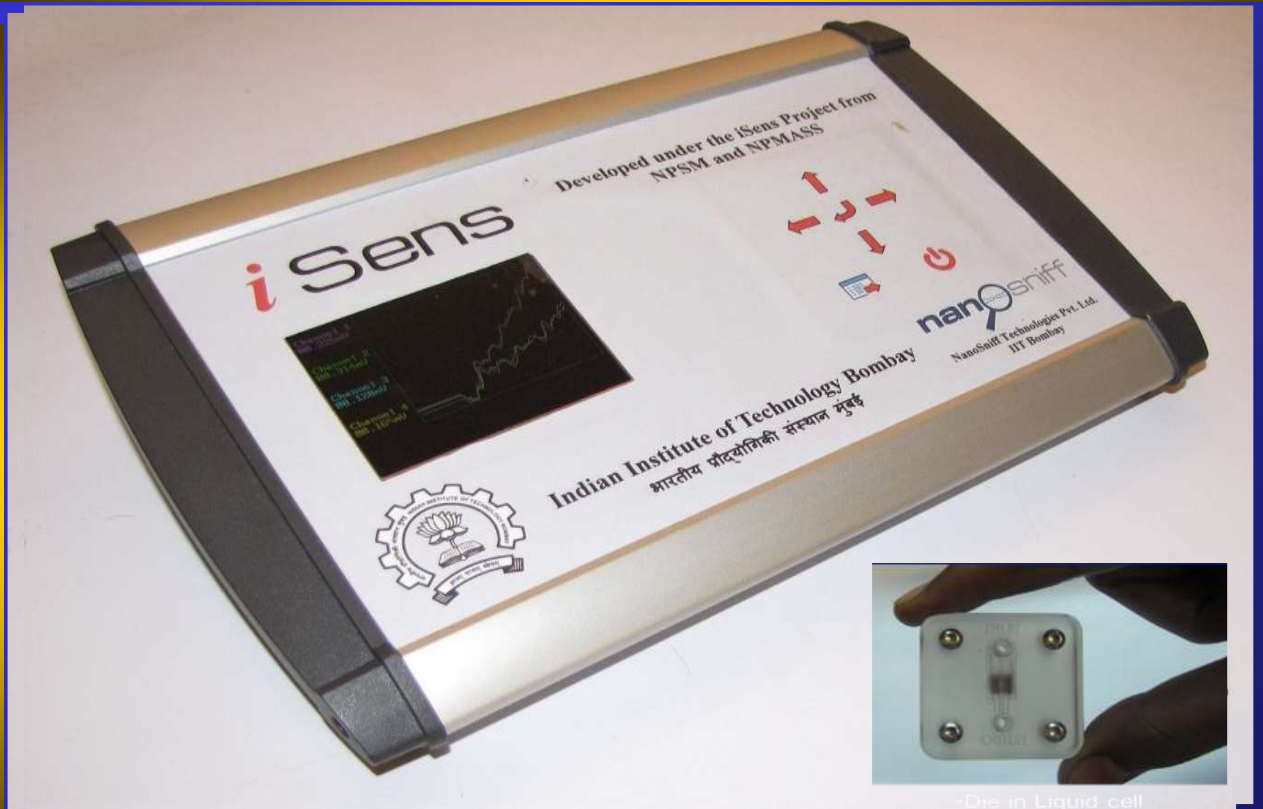
Ver-2 for Hospital Trials: iSens Working prototype built jointly with NanoSniff Technologies Pvt. Ltd.
