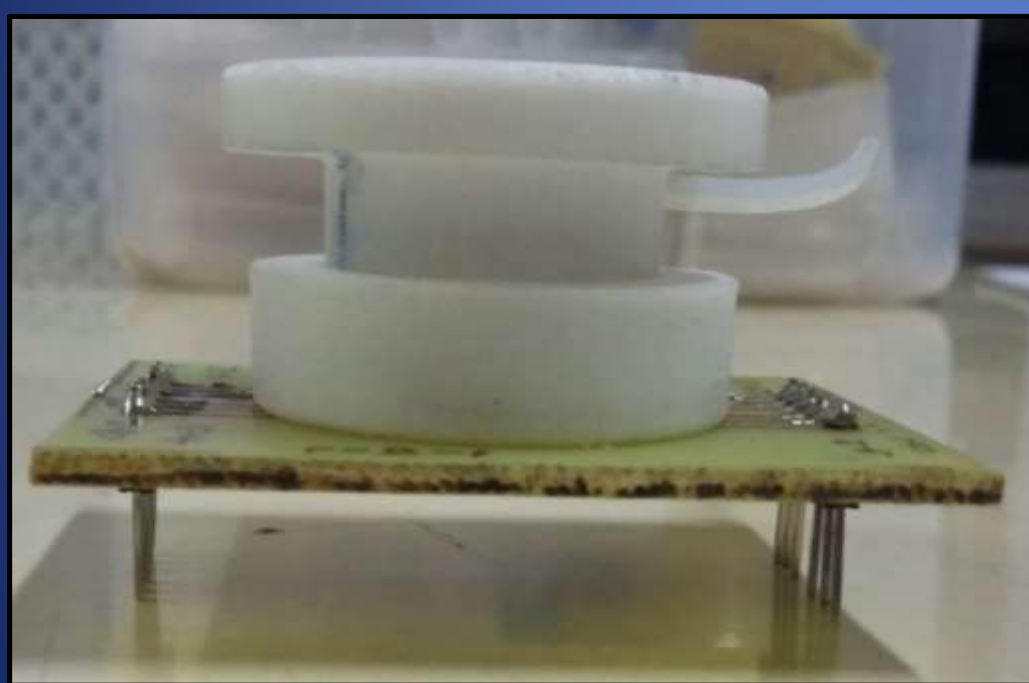
4-Channel Sensor cartridge with flow cell assembly
