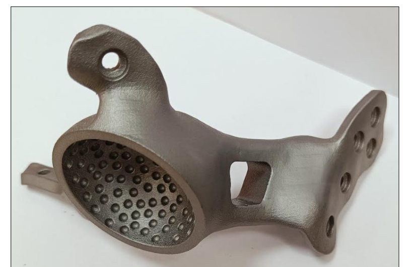
Customised implant for acetabular cup fixation
