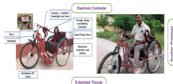
Control Module integrated with e-tricycle
