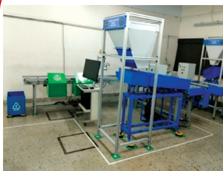
AI-enabled NIR optical sorter system
