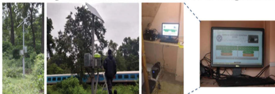
Seismic Sensing Node and Control and Command Server for alert generation
