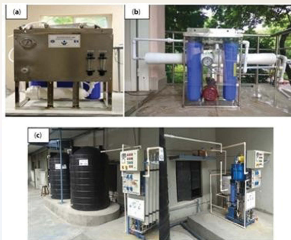
Figure Indigenous RO/NF systems developed by CSIR-IICT for defluoridation of ground water and surface water purification. Source: S. Sridhar et al. (ed.) Membrane Processes, (1- 36) © 2019 Scrivener Publishing LLC
