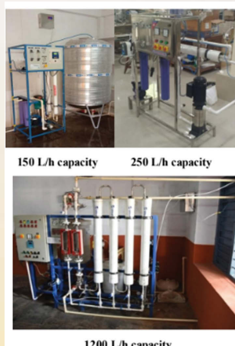
Figure Indigenous RO/NF systems developed by CSIR-IICT for defluoridation of ground water and surface water purification. Source: S. Sridhar et al. (ed.) Membrane Processes, (1- 36) © 2019 Scrivener Publishing LLC
