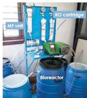
Pilot scale bio-physical unit for treating perchlorate contaminated ground water.
