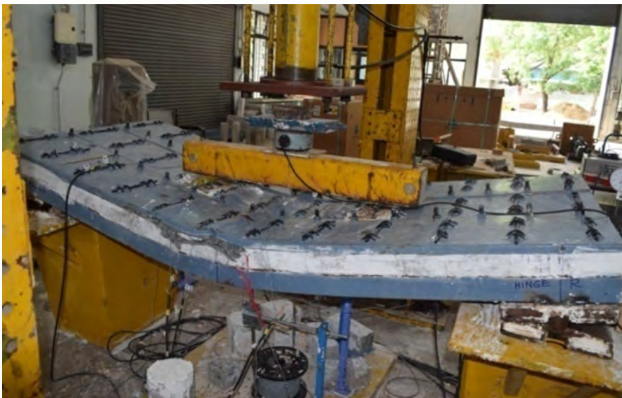
Flexural testing of i-LSCC panel
