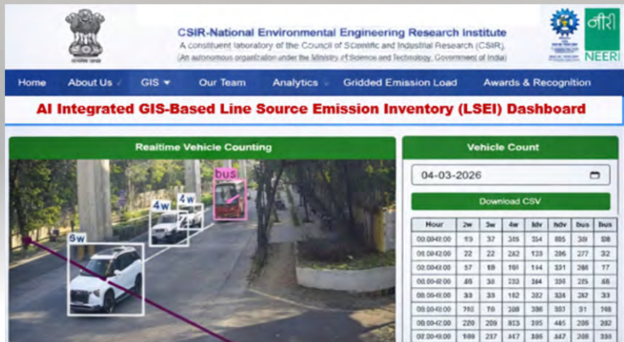
Sample of how the AI dashboard identifies and counts different vehicle categories
