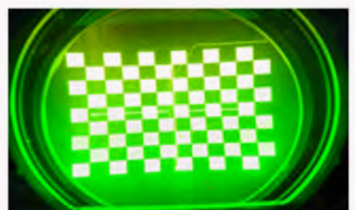
HUD Symbology during Night-Stroke in Raster Mode
