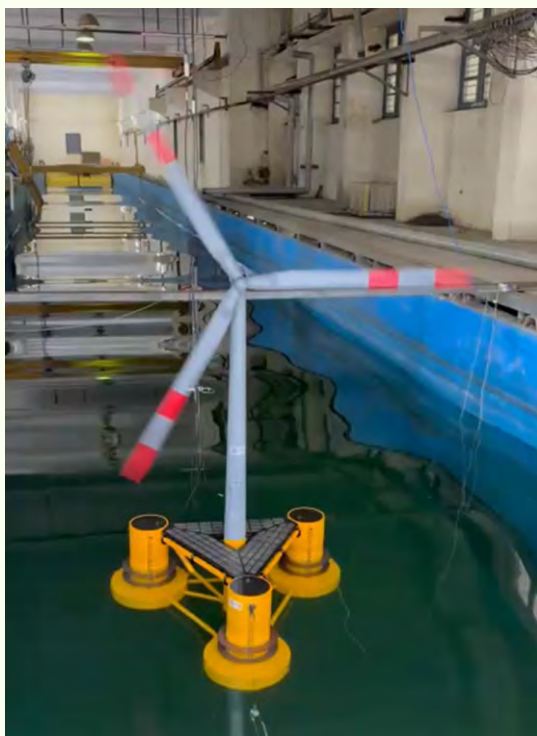
Floating offshore hybrid energy platform configurations at CSIR-SERC
