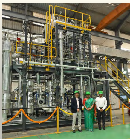
CSIR-NCL's 250 kg/day Methanol-to-DME Pilot Plant, developed using a patented indigenous catalyst.
