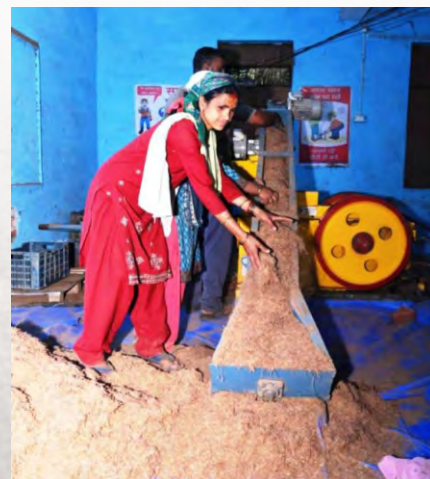
Pine needle briquetting machine being operated by the trained women of "Ujjwal Mahila Samooh" under the guidance of CSIR-IIP
