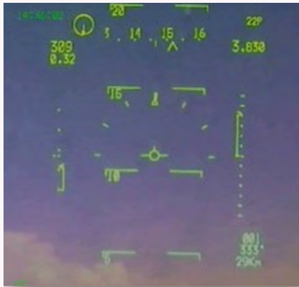
HUD Symbology Through CSIR-CSIO Developed HUD on Beam Combiner
