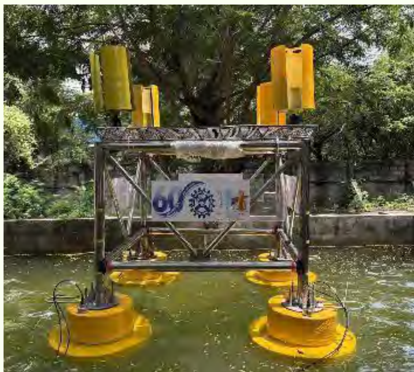
Floating offshore hybrid energy platform configurations at CSIR-SERC
