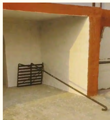
Drag Rod for taking the soft coke out from the oven
