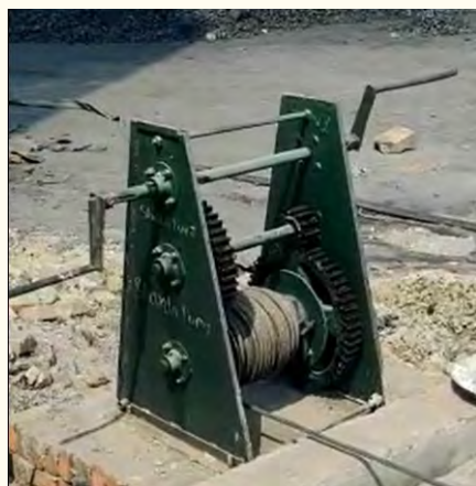
Which used for pulling the soft coke out from the oven through drag rod.
