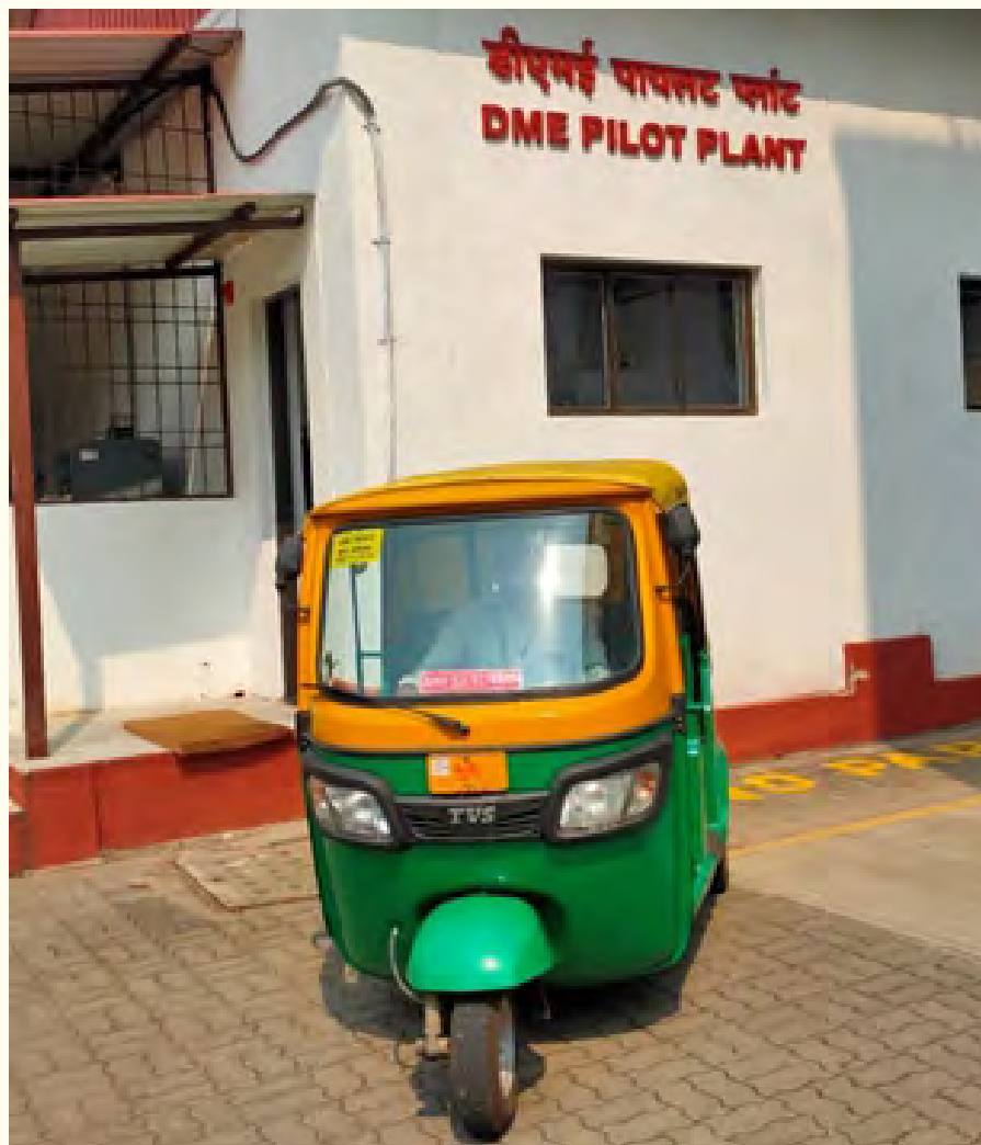
ARAI-tested DME-LPG three-wheeler at CSIR-NCL.
